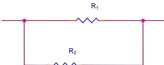
$$\frac{1}{R_e} = \frac{1}{R_1} + \frac{1}{R_2} + \frac{1}{R_3} + \dots + \frac{1}{R_N}$$
