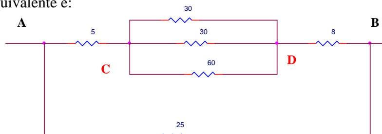
$$\frac{1}{R_2} = \frac{1}{30} + \frac{1}{30} + \frac{1}{60} \Rightarrow \frac{1}{R_2} = \frac{5}{60} \Rightarrow R_2 = 12\Omega$$
